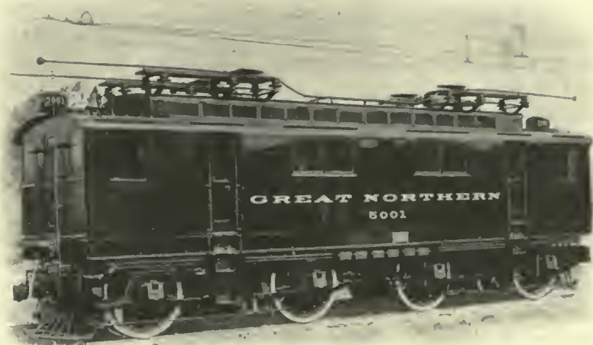
FIG. 542. ELECTRIC LOCOMOTIVES. Locomotive for Three-Phase Overhead Contact Operation, Great Northern Railway.
